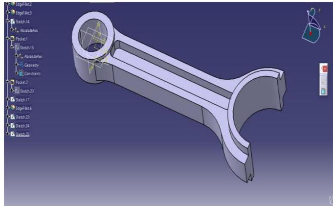
Figure 1. 3D solid model of Connecting Rod
