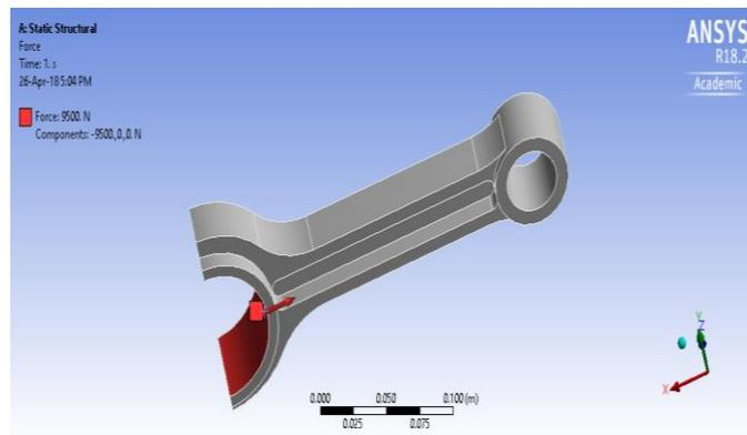
Figure 5. Compressive Loading on Connecting Rod
