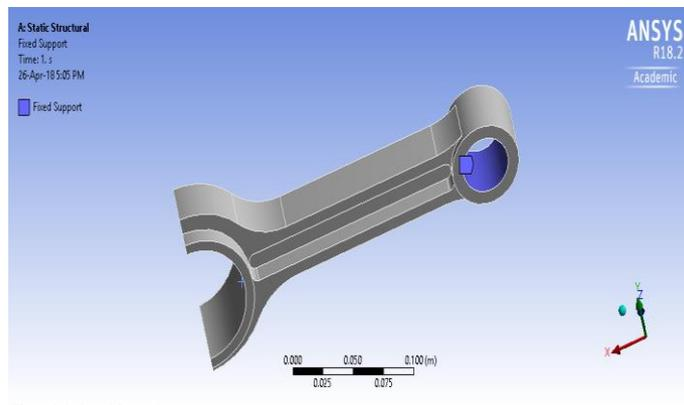
Figure 3. Boundary Condition on Connecting Rod
