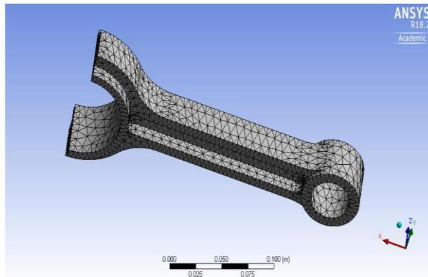
Figure 2. 3D meshed model of connecting rod
