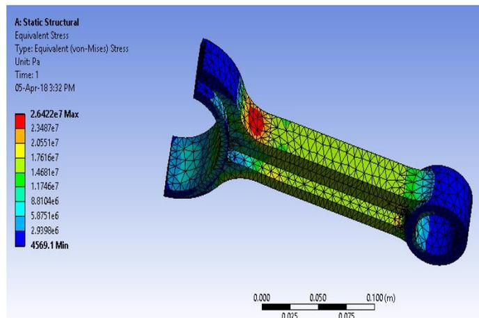
Figure 6. Stress generated at fillet radius on connecting rod
