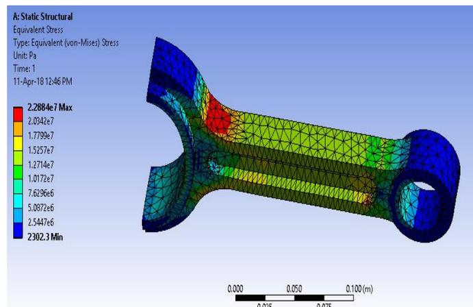
Figure 8. Stress generated at groove length on connecting rod
