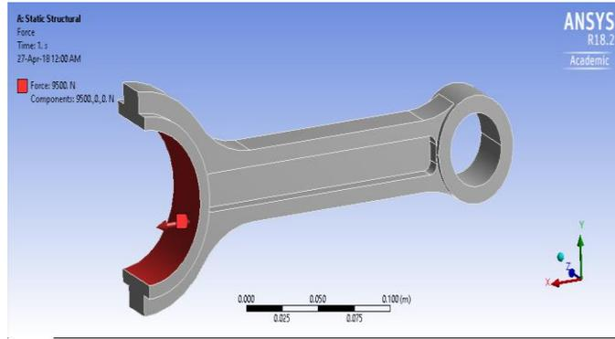
Figure 4. Tensile Loading on Connecting Rod
