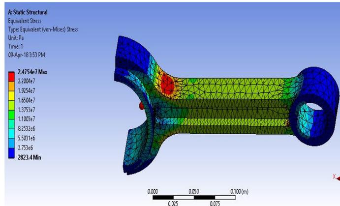
Figure 7. Stress generated at groove depth on connecting rod
