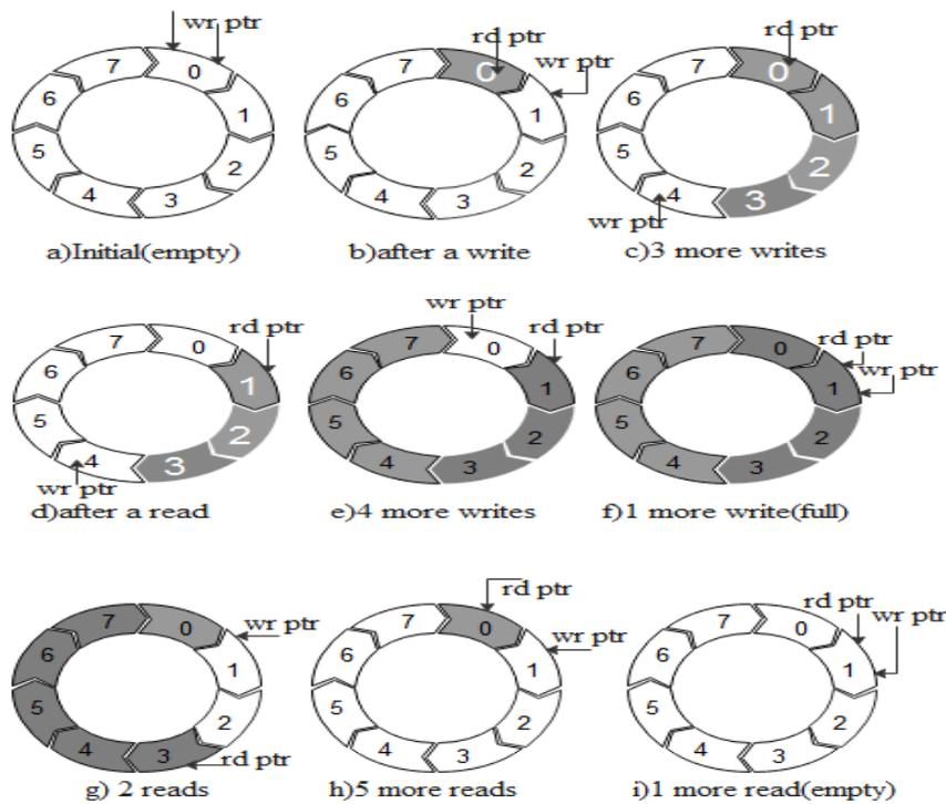
Fig. 1. Implementation of FIFO using circular buffer
