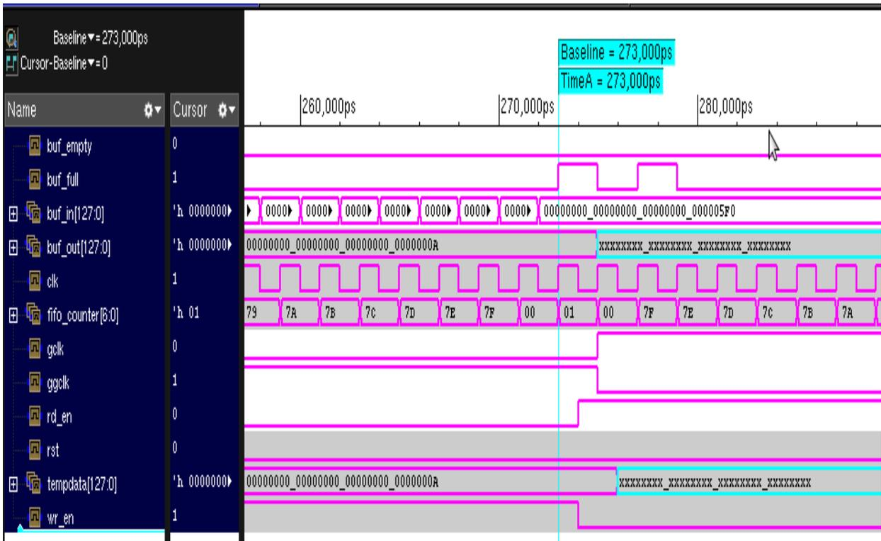
**Fig.6. Simulation of 128 x 128 FIFO buffer in empty state with pipeline**
