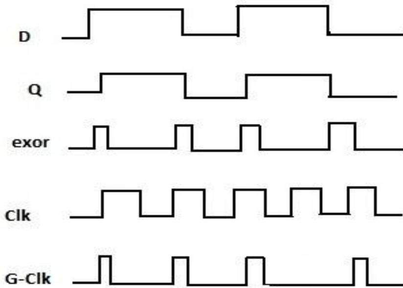
Fig. 4 Simulation waveforms for clock gating D flip flop
