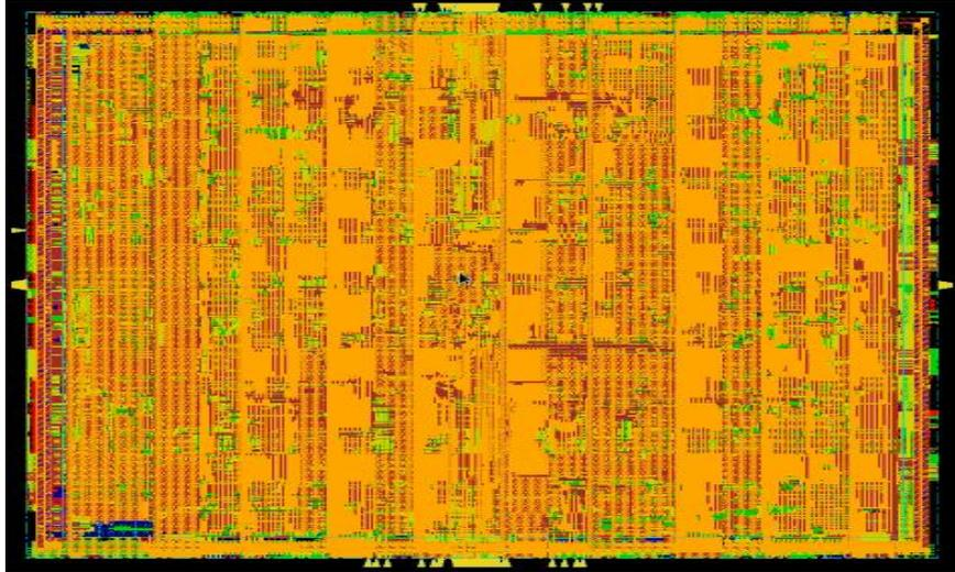
**Fig.9. Metal fill of 128 x 128 bit synchronous FIFO buffer**
