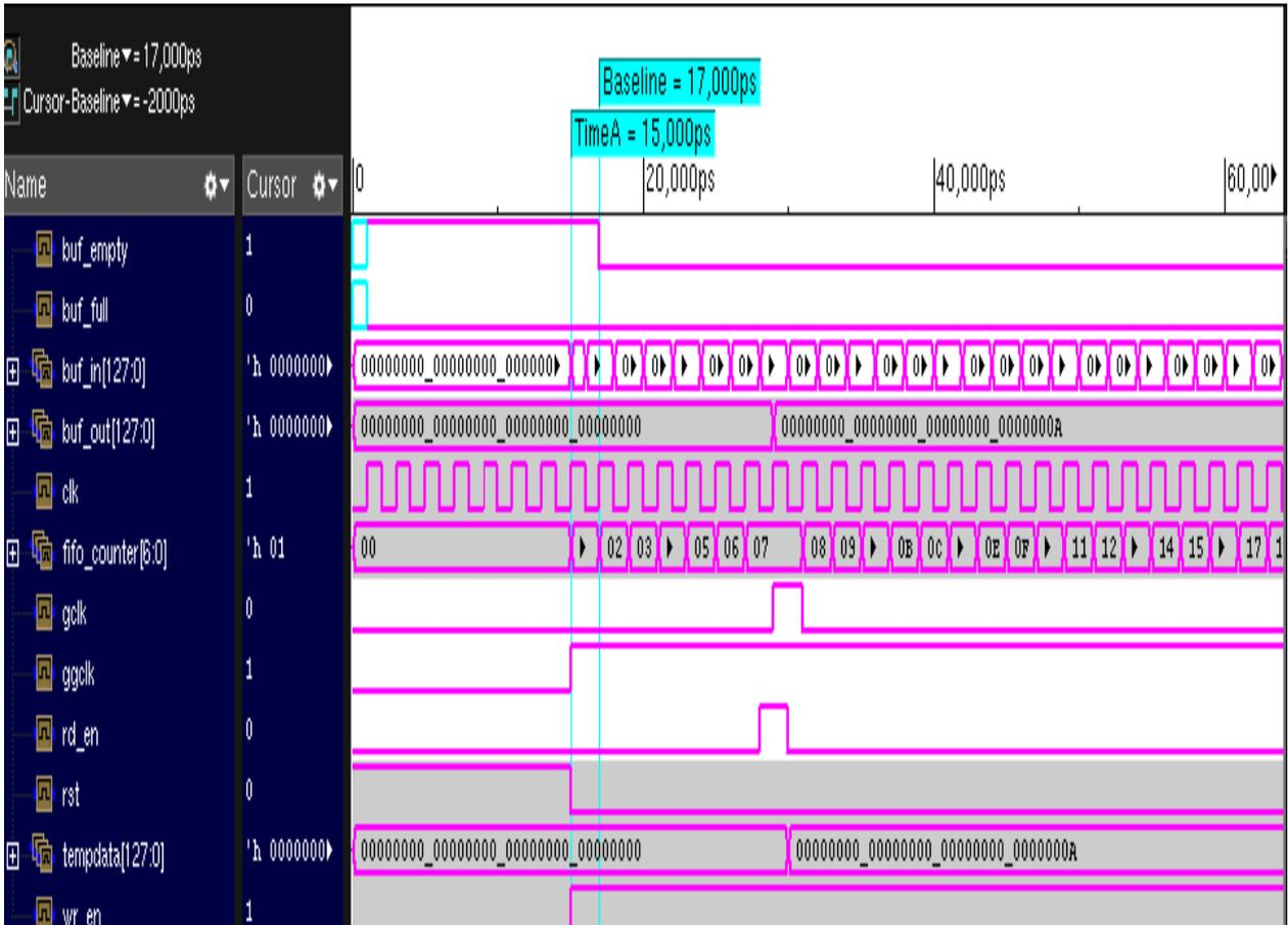
**Fig.5. Simulation of 128 x 128 FIFO buffer in empty state without pipeline**
