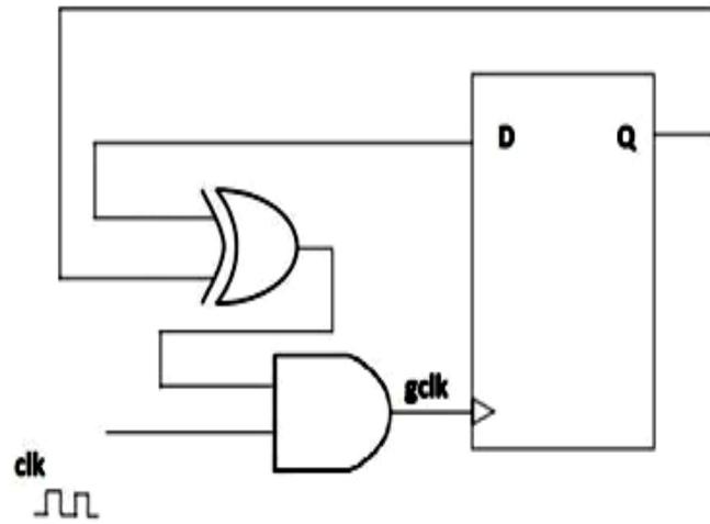
Fig. 3. Latch free clock gating D flipflop
