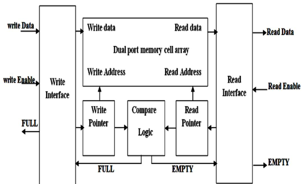
Fig. 2. Block diagram Synchronous FIFO with dual ported memory cell array
