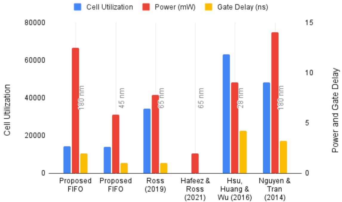
Fig. 8. Implementation of area, delay and power parameters for conventional and proposed synchronous FIFO
