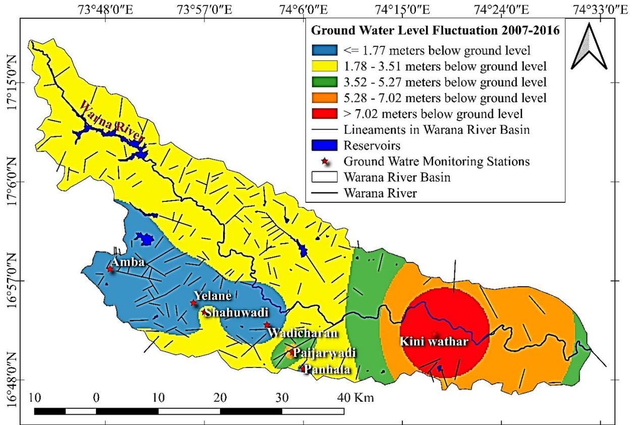
**Figure 7.** Groundwater Table Fluctuation Map of Pre and Post Monsoon season for 10 years (2007-2016) based on groundwater monitoring stations in the Warana River Basin
