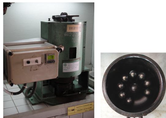
Figure 1. Ball-race Hardgrove machine.
