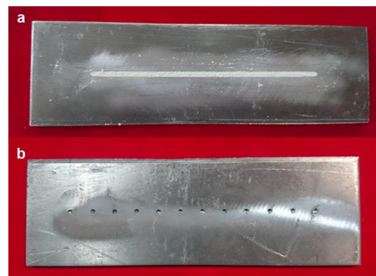
Figure 1. Provision to fill reinforcement particles: a) Rectangular groove; b) Linear array of cylindrical holes
