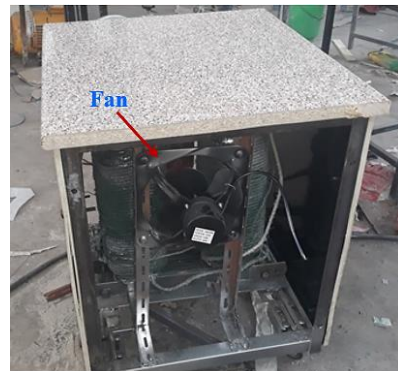
Figure 5. Air cooling system
