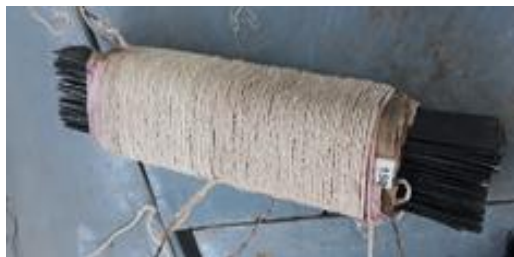
Figure 3. Primary winding of right limb of a transformer
