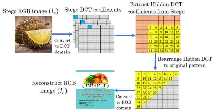
Figure 6. Diagram for decoding process
