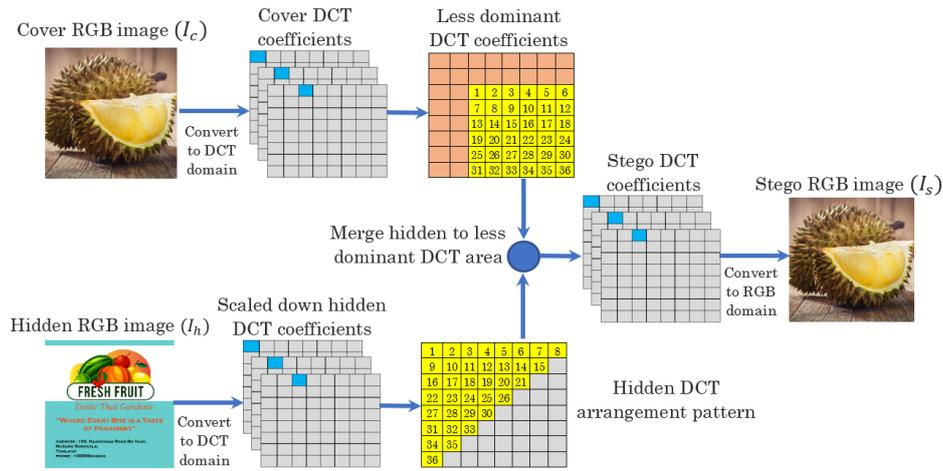
Figure 5. Diagram for encoding process
