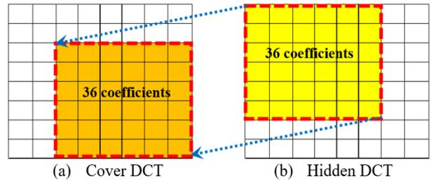
Figure 3. Selection area of cover and hidden DCT coefficients in embedded process
