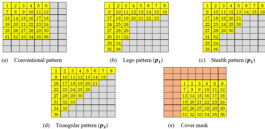
Figure 4. DCT arrangement patterns for hidden (a – d) and cover (e) images
