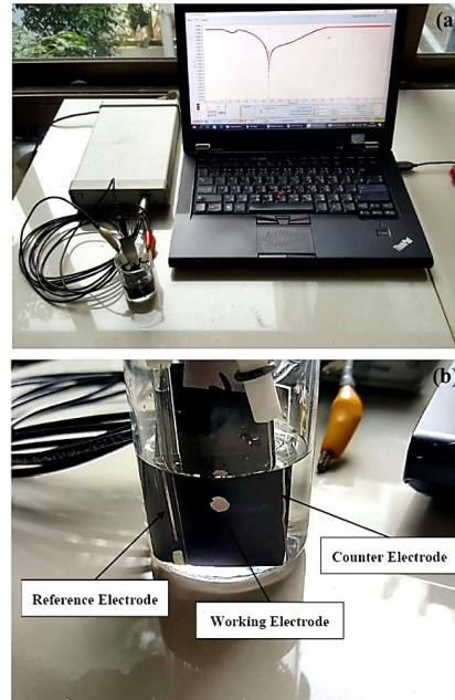
Figure 1. Potentiodynamic polarization test equipment: (a) DY2300 potentiostat program and DY2322 potentiostat, and (b) experimental electrode apparatus parts
