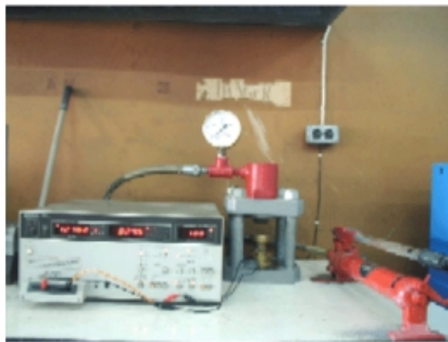
Figure 4. Experimental set up for studying the effect of high stress on dielectric properties of PMN-PZT.
