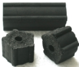
Figure 6. Photo showing the extruded fuel from the experiments.
