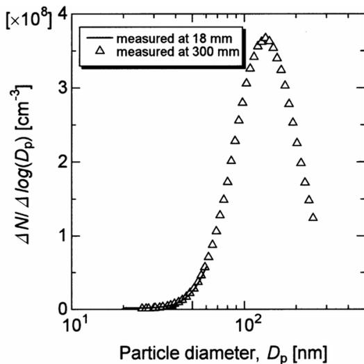
Figure 11. Particle size distribution measured with the ACLDMA when  $L = 18$  and  $300$  mm (Seol *et al.*, 2002).
