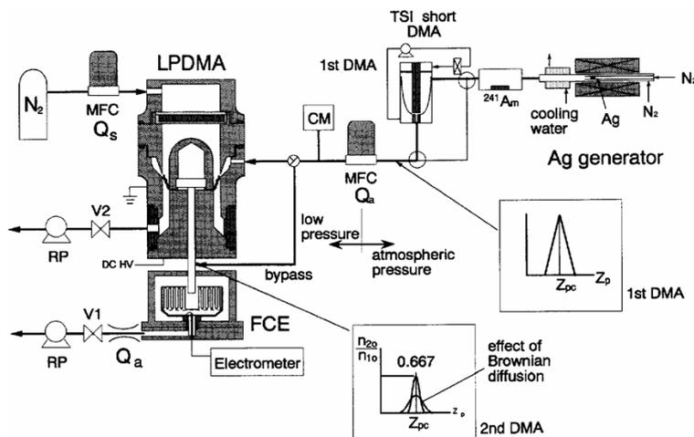
Figure 8. Experimental system for calibration of LPDMA (Seto *et al.*, 1997).
