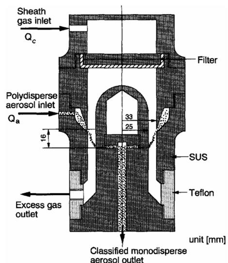
Figure 7. Schematic diagram of the LPDMA developed by Seto *et al.* (1997).
