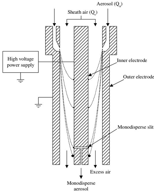
Figure 1. Basic principle of a general DMA.
