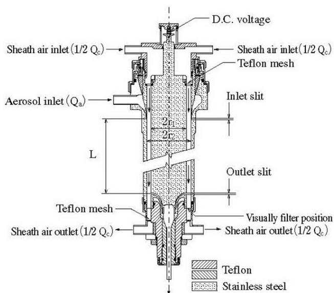
Figure 14. Schematic of the large flow annular-type DMA (Koyama et al., 2007).
