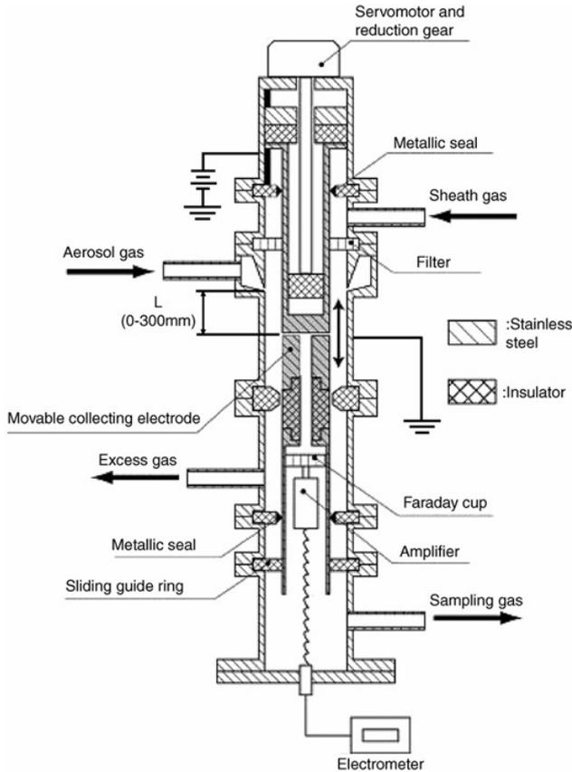
Figure 10. Schematic of an adjustable-column length DMA (ACLDMA) (Seol *et al.*, 2002).
