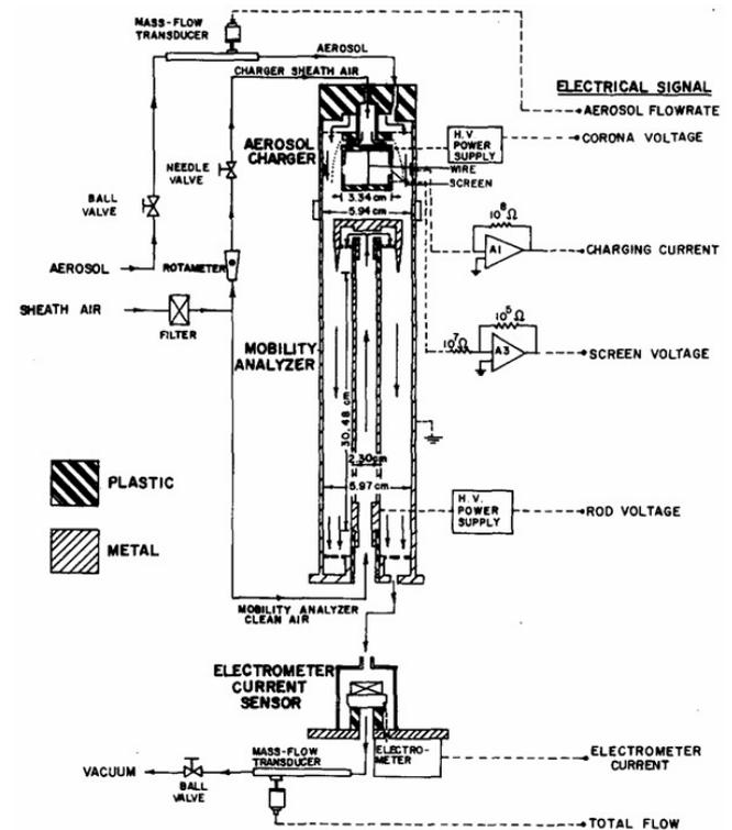
Figure 2. The electrical aerosol analyzer developed by Liu and Pui (1975).
