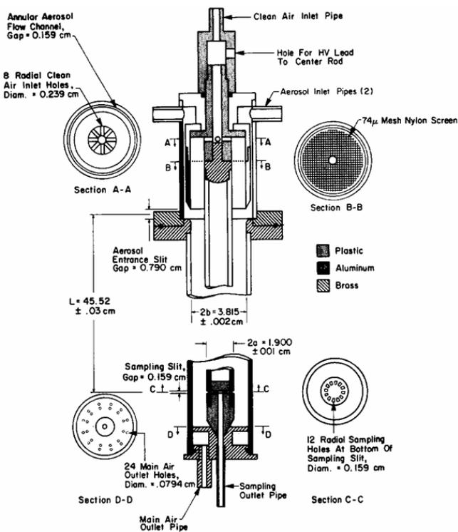
Figure 3. The mobility analyzer developed by Knutson and Whitby (1975).
