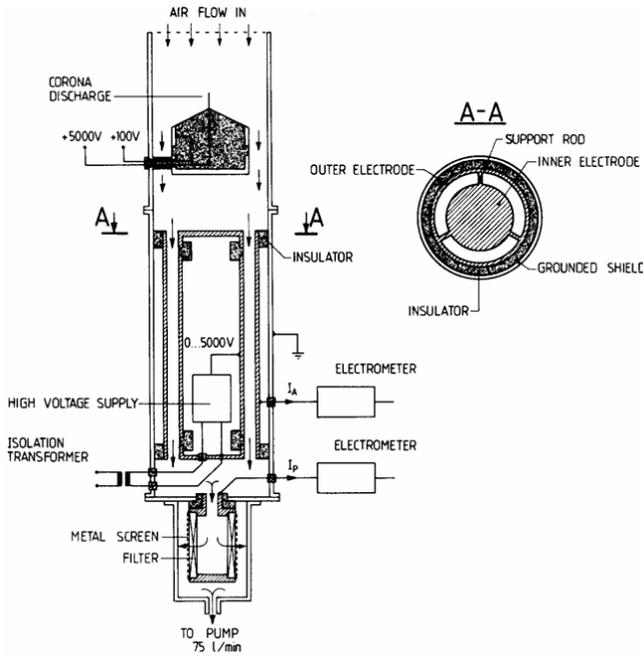
Figure 5. Schematic diagram of the analyzer developed by Lehtimäki (1987).
