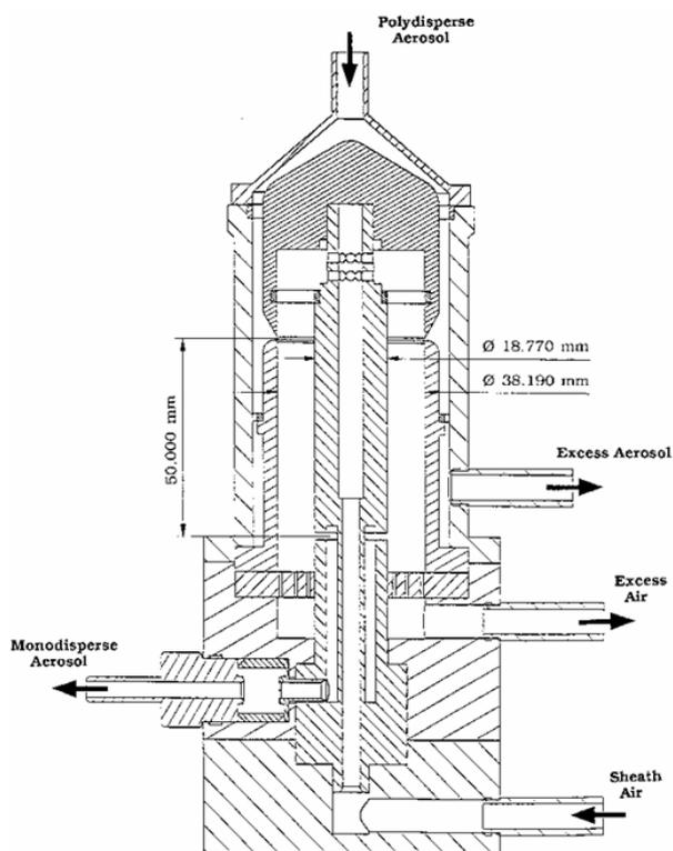
Figure 9. Schematic diagram of the Nano-DMA developed by Chen *et al.* (1998).
