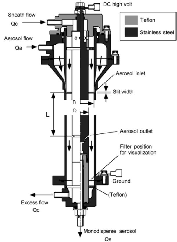
Figure 12. Schematic of the LDMA-FCE system (Shimada *et al.*, 2005).
