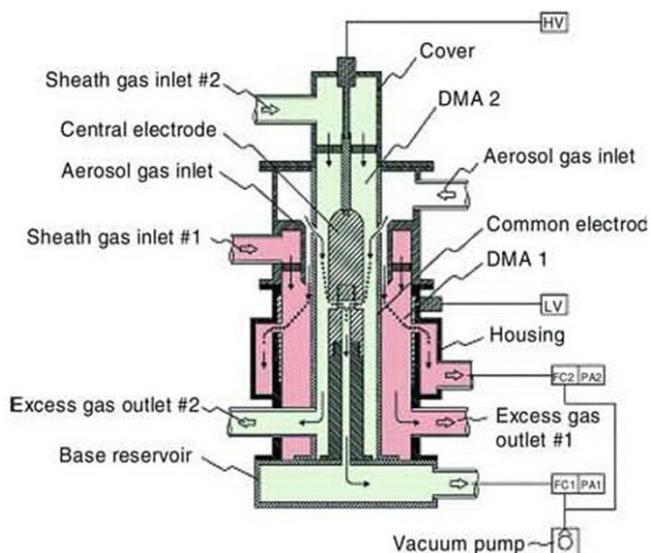
Figure 18. Schematic of the new dual-type DMA (Takeuchi *et al.*, 2005).
