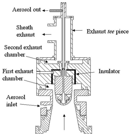
Figure 13. Schematic of the Nano-DMA developed by Rosser and Fernandez de la Mora (2005).
