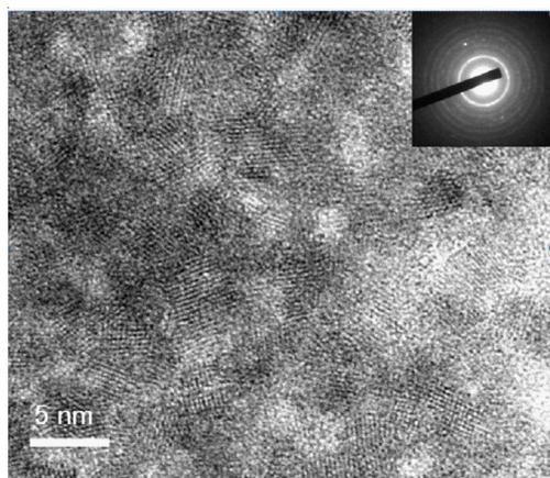
Figure 5. TEM image of the specimen taken from the titanium alkoxide precursor solution. A selected area electron diffraction pattern corresponds to anatase  $\text{TiO}_2$ .
