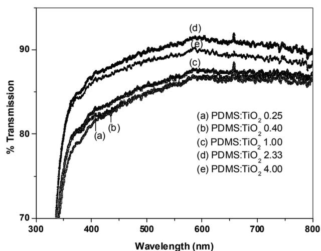
Figure 7. Transmission spectra of as-prepared hybrid films having various ratios of PDMS and  $\text{TiO}_2$ .
