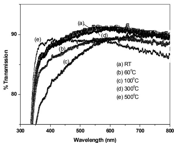
Figure 6. Transmission spectra of the as-prepared hybrid film, and the films heated at 60-500°C. The films were prepared from the precursor containing volume ratio of PDMS:  $\text{TiO}_2$  of 2:1.
