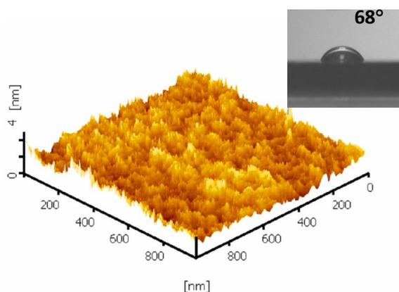
Figure 1. A 3D AFM topographical image of bare glass substrate. The bare surface exhibited water contact angle of 68 degrees.
