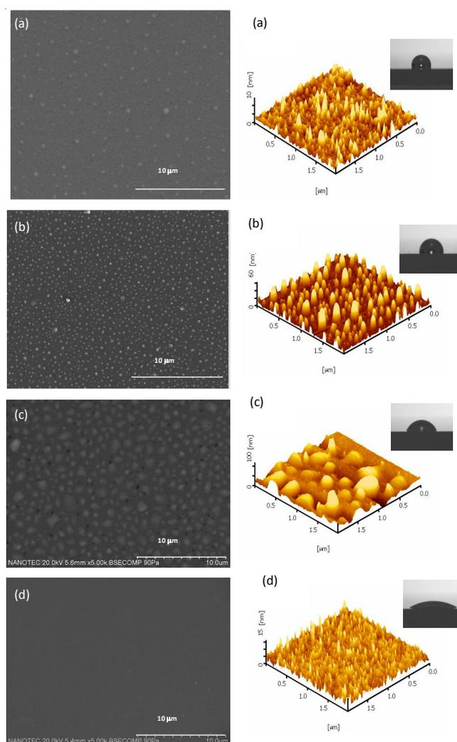
Figure 3. SEM and 3D AFM topographical images of the hybrid films surface on the glass substrate: (a) as-prepared, (b) heated at 100°C, (c) heated at 300°C and (d) heated at 500°C.
