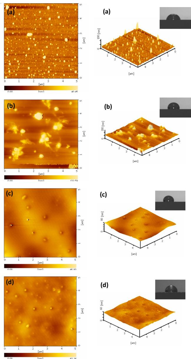
Figure 4. 2D and 3D AFM images of the hybrid surfaces having the PDMS/TiO<sub>2</sub> volume ratio of (a) 0.25, (b) 1.00, (c) 2.33 and (d) 4.00 at heat-treatment temperature of 60°C.
