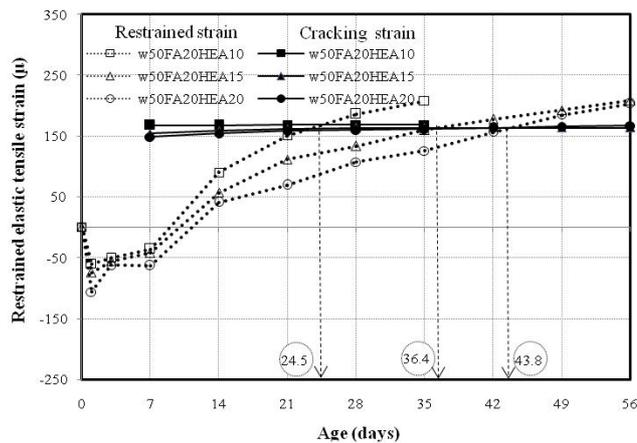
(e) The restrained elastic tensile strain without tensile creep and cracking strain of expansive concrete (Hyper expansive additive using 20% fly ash)
