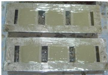
(d) The equipment for casting of samples for restrained compressive strength measurement
