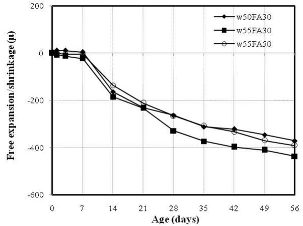
(b) Free expansion/shrinkage of fly ash concrete
