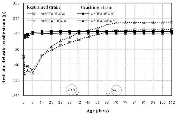
(c) The restrained elastic tensile strain without tensile creep and cracking strain capability of expansive concrete (Normal expansive additive)
