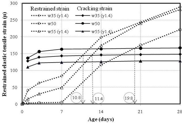
(a) The restrained elastic tensile strain without tensile creep and cracking strain capability of cement- only concrete
