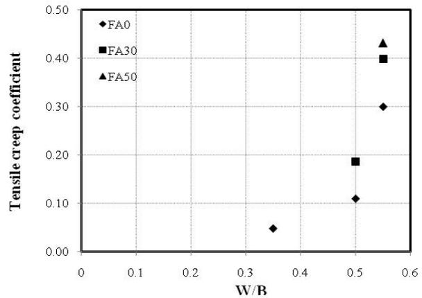
Figure 5. Relationship between tensile creep coefficient and ratio water to binder
