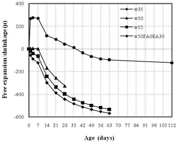
(a) Free expansion/shrinkage of concrete without fly ash
