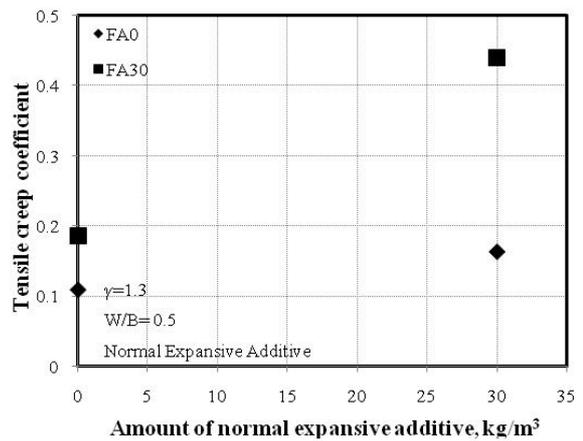
(a) Concretes with normal expansive additive (EA)
