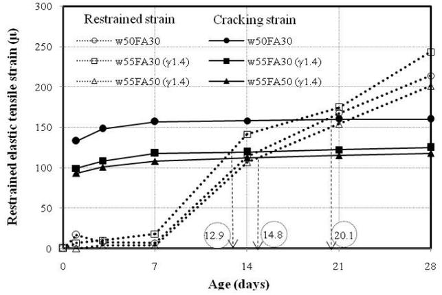
(b) The restrained elastic tensile strain without tensile creep and cracking strain capability of fly ash concrete
