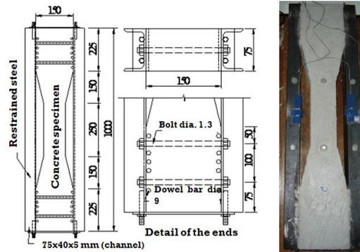
(a) Externally restrained specimen (unit: mm)
