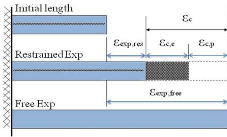
(a) Expansion mechanism of expansive concrete under restraint
