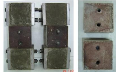
(e) Restrained compressive strength samples before and after removing restraining steel
