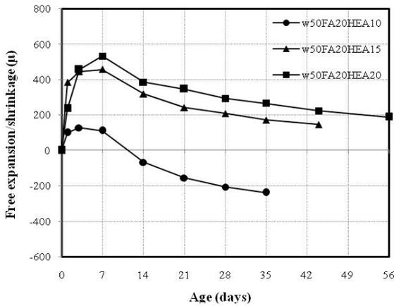
(c) Free expansion and shrinkage of expansive concrete using 20% fly ash
