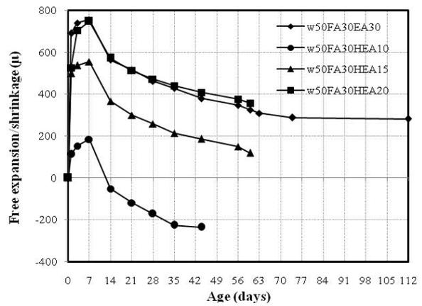
(d) Free expansion and shrinkage of expansive concrete using 30% fly ash
