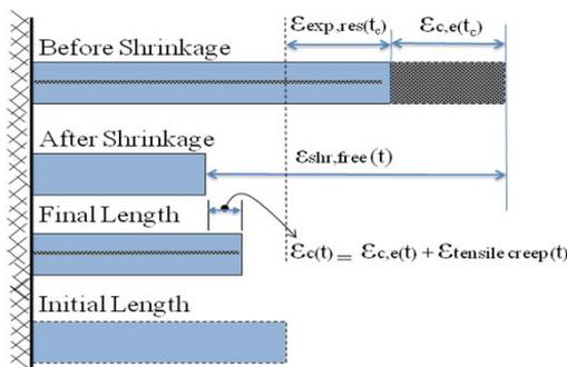
(b) Shrinkage mechanisms of expansive concrete under restraint
