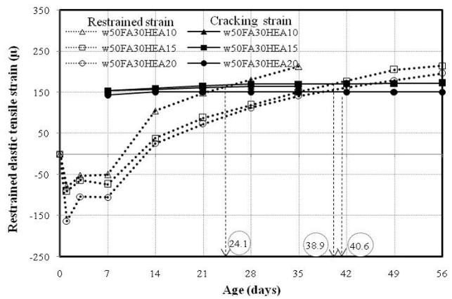
(d) The restrained elastic tensile strain without tensile creep and cracking strain capability of expansive concrete (Hyper expansive additive using 30% fly ash)
