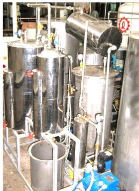
Figure 5. Photograph of evaporator.
