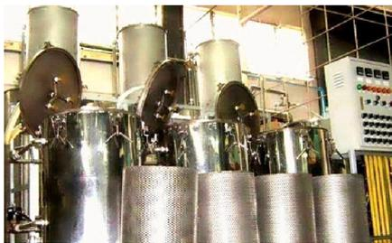
Figure 4. Photograph of continuous extractor.
