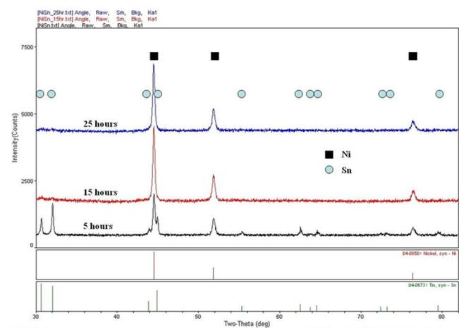
Figure 1. X-ray diffraction patterns of the Ni+Sn powders milled for different times.
