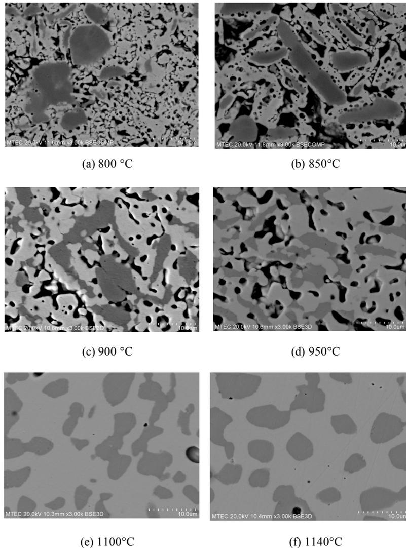
Figure 5. Eutectic Ni-Sn alloy resulted from 10 minute-heating of milled Ni-Sn powders at temperatures of (a) 800°C, (b) 850°C, (c) 950°C, (d) 950°C, (e) 1100°C, and (f) 1140°C.
