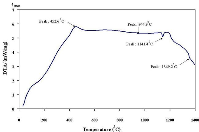
Figure 3. Differential thermal analysis of Ni+Sn powders milled for 25 hours.
