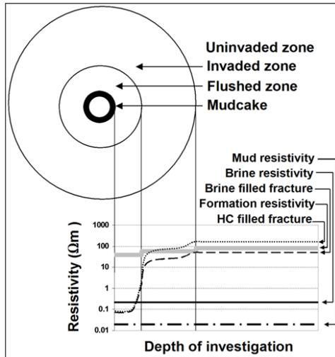
Figure 4. Schematic diagram of the borehole environment including mud cake, flushed zone, invaded zone, and uninvaded zone, and a qualitative transition profile of the electrical resistivity (ohm m) when a fracture is present (hydrocarbon or brine filled) of a sandstone formation with porosity <5%.
