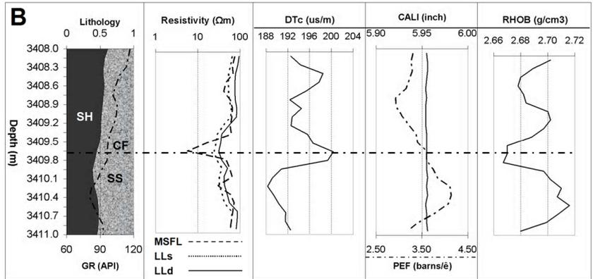
Figure 7. Fracture analyses in the depth interval between 3408.0 m and 3411.0 m.
