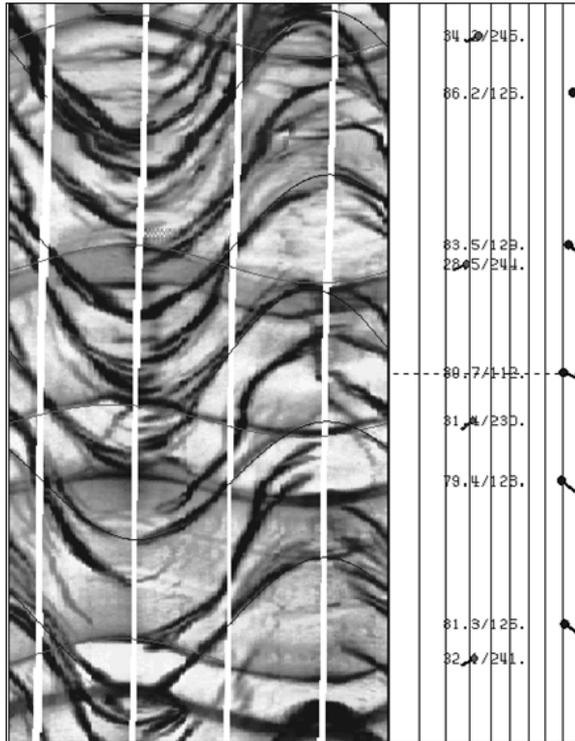
Figure 2. Example of an FMI image with dipping fractures relative to the borehole axis as sinus curves. On the right showing the processed data with dip direction and dip angle (after HEF, 2011). Note that the image is not from this study.
