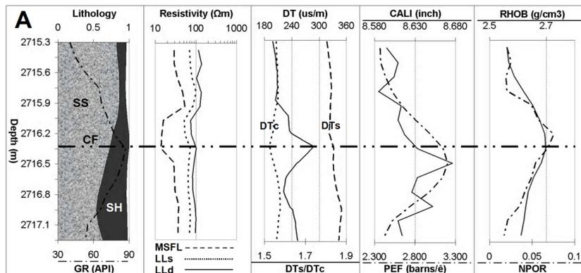
Figure 6. Fracture analyses in the depth interval between 2715.3 m and 2717.1 m.
