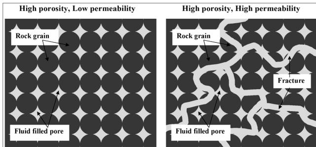
Figure 1. Fracture porosity increases permeability and fractures as fluids path way contribute to permeability. Left: without fracture; Right: with fractures.
