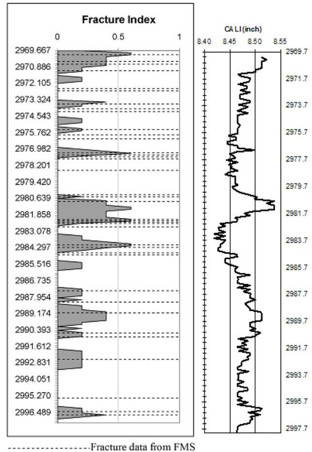
Figure 10. Correlation of the fracture index with fractures data from FMS in the depth interval between 3589.2 m and 3591.3 m.
