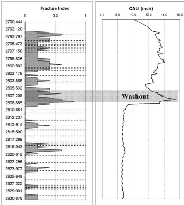
Figure 9. Correlation of the fracture index with fractures data from FMS in the depth interval between 2790.444 m and 2830.678 m.
