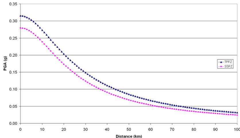
Figure 8. PGA versus epicentral distance of the TPFZ and the SSFZ calculated from their surface rupture lengths using the Sadigh *et al.* (1997) relationship. See text for detailed explanation.
