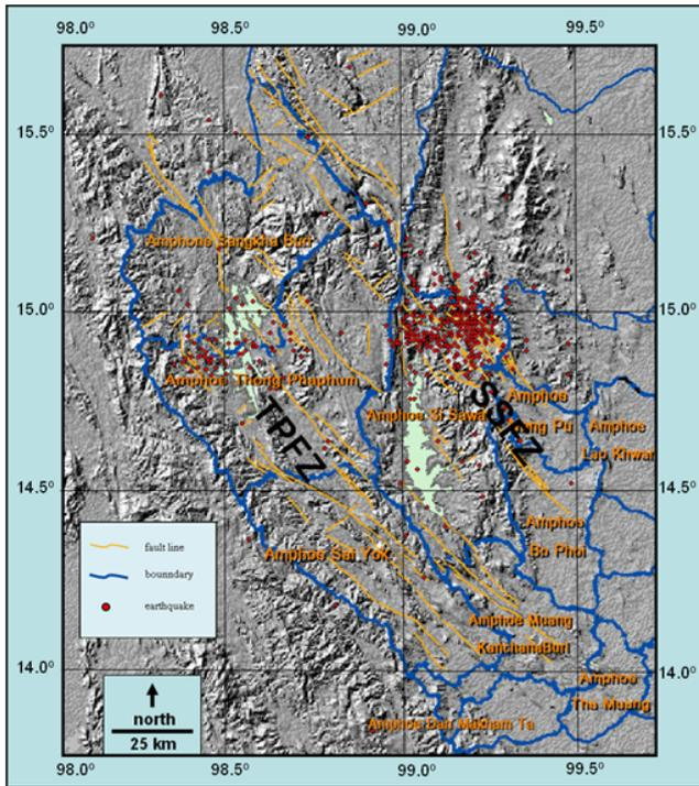
Figure 2. Seismicities in Kanchanaburi, western Thailand (red dots) overlain on the DEM. Yellow lines are the probable locations of the active faults. Blue lines are political boundaries.
