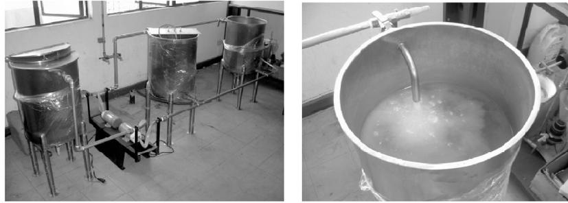
Figure 9. Pilot scale CIP plant.
