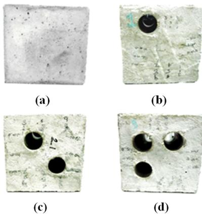
Figure 5. Samples for classification of the number of defects: (a) Non-defective specimen, (b) One defect specimen (c) Two defects specimen, and (d) Three defects specimen.
