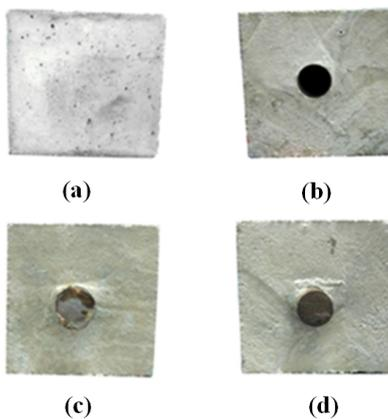
Figure 6. Samples for identification of defect materials: (a) Non-defective specimen, (b) Specimen with air void, (c) Specimen with steel rod, and (d) Specimen with wood rod.
