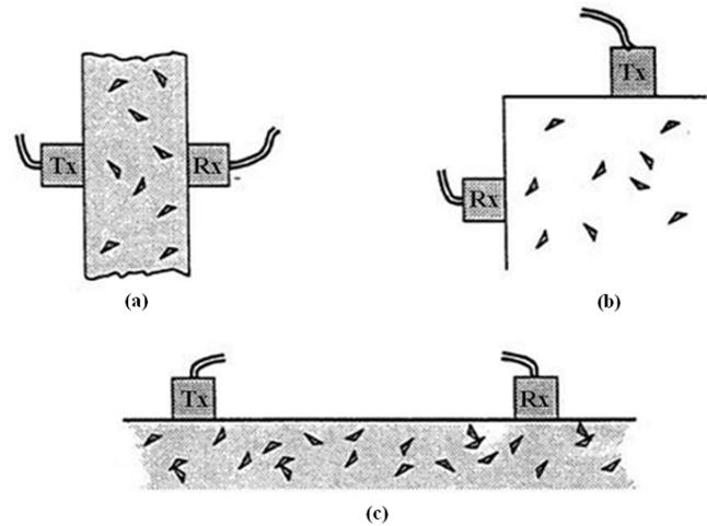
Figure 7. Ultrasonic pulse velocity measurement methods: (a) Direct measurement, (b) Semi-direct measurement, and (c) Indirect measurement.
