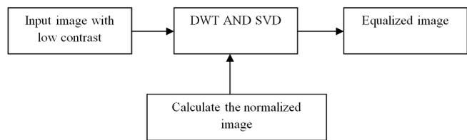
Figure 2. Fingerprint image enhancement method using discrete wavelet transform
