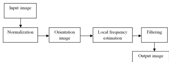
Figure 3. Block of the fingerprint image enhancement
