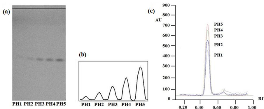
Figure 2. The TLC pattern (a) for the phyllanthin standard at concentrations of 1, 2, 5, 7.5, and 10  $\mu\text{g}/\text{spot}$  (PH1 - PH5). The TLC chromatogram was generated through (b) the TLC-image analysis and (c) the TLC-densitometric method.
