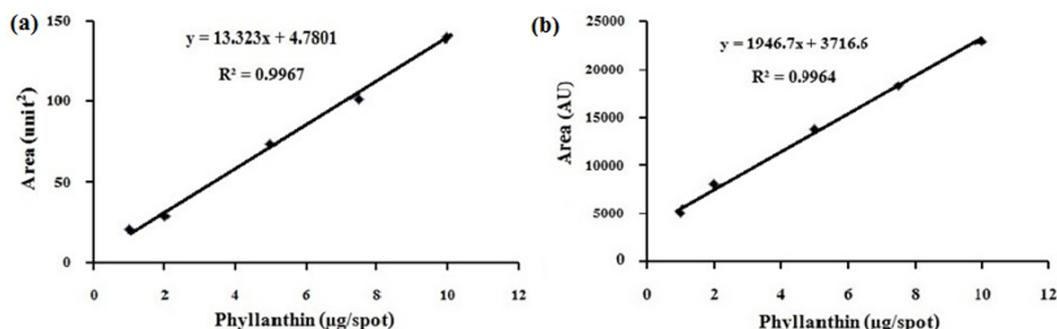
Figure 3. Standard curve for the peak area and phyllanthin concentrations from (a) TLC-image analysis ( $\text{unit}^2$ ) and (b) TLC-densitometry (AU) ( $n = 6$ ).
