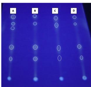
Figure 2. TLC chromatograms of wax from banana leaves: (A), (B) - BNT, before and after decolorization; (C), (D) BNS, before and after decolorization respectively.
