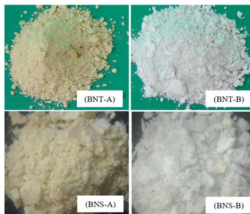
Figure 1. Epicuticular wax extracted from banana leaves, BNT and BNS; (A) before decolorization, (B) after decolorization.
