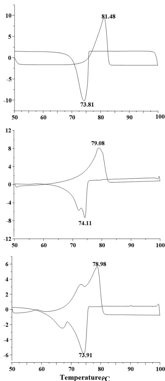
Figure 4. DSC thermograms wax from banana waxes; BNT-upper, BNS-middle and carnauba wax-lower.
