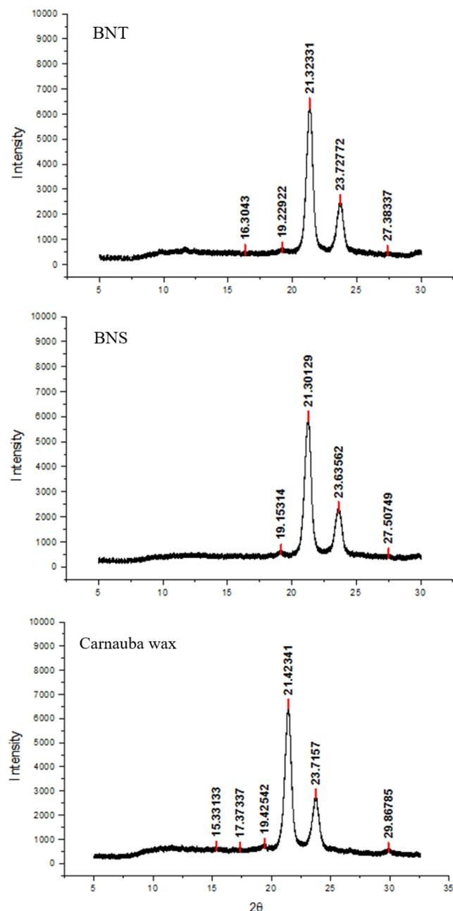
Figure 5. X-ray powdered diffractograms of wax from banana leaves: BNT, BNS and carnauba wax.
