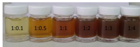
Figure 1. Synthesis of AgNPs using various concentration ratios of \text{AgNO}_3 (mM) and G. glabra root extract (mg/ml) as 1:0.1, 1:0.5, 1:1, 1:2, 1:3, and 1:4. The image shows solutions after heating for 2 min with color changes upon formation of the AgNPs.
