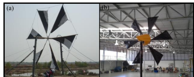
Figure 1. Thai sail windmill (TSW) (a) Conventional TSW (b) DTSW model.
