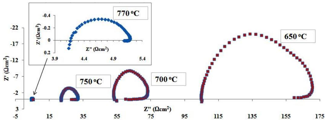
Figure 7. AC impedances spectra of symmetrical cells (BYCF|GDC<sub>10</sub>|BYCF) at temperature 650, 700, 750 and 770 °C.
