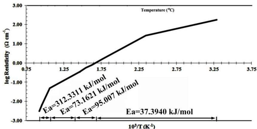
Figure 6. Electrical conductivity of the  $\text{Ba}_{0.08}\text{Y}_{0.04}\text{Co}_{2.5}\text{Fe}_{0.09}\text{O}_{4.8}$  composite at different temperatures.
