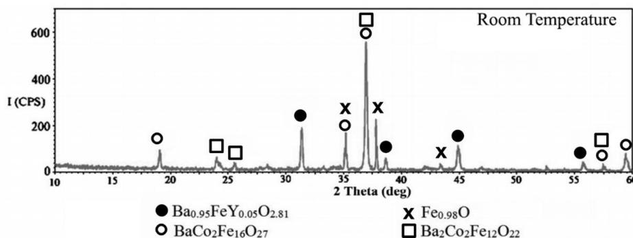
Figure 4. XRD pattern for  $\text{Ba}_{0.08}\text{Y}_{0.04}\text{Co}_{2.5}\text{Fe}_{0.09}\text{O}_{4.5}$  at room temperature.
