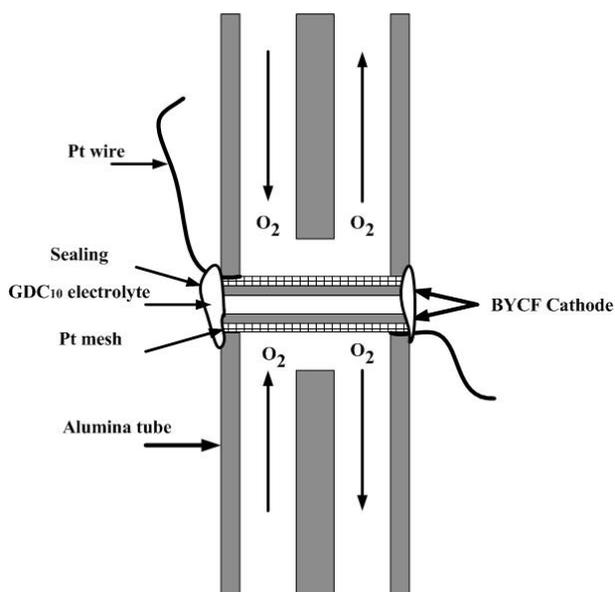
Figure 3. Sample holder for AC impedance spectroscopy measurement.
