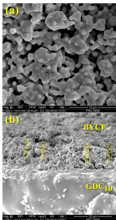
Figure 2. SEM micrographs: (a) fractured surface of BYCF+20% GDC<sub>10</sub> and (b) BYCF-GDC<sub>10</sub> interfaces.
