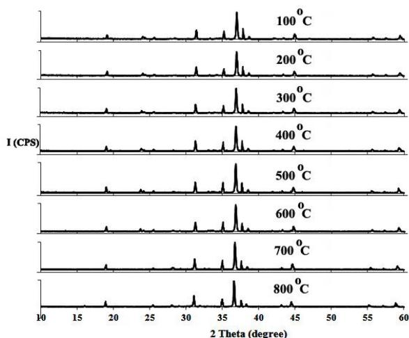
Figure 5. XRD patterns of  $\text{Ba}_{0.08}\text{Y}_{0.04}\text{Co}_{2.5}\text{Fe}_{0.09}\text{O}_{4.8}$  at elevated temperatures.
