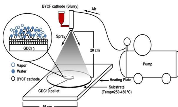
Figure 1. Principle of the spray pyrolysis process.
