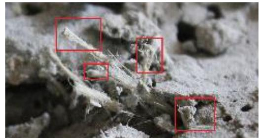
(c) Pull-out failure of aramid fiber
