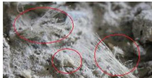
(b) Rupture failure of aramid fiber
