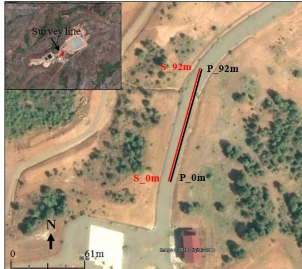
Figure 3. The P- and S-wave spread lines at the study area (Google Earth, 2016).
