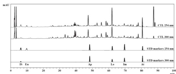
Figure 2. HPLC Chromatogram of CTL detection at UV 254 nm and at UV 300 nm compared with standard markers including eurycomanone (Eu), apigenin (Ap), loureirin A (Lo), imperatorin (Im) and atractylodin (At).
