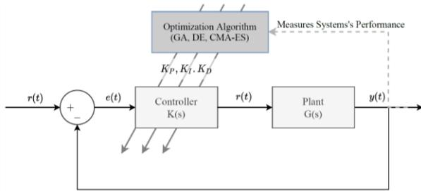
Figure 2. Optimization process to tune the PID controllers
