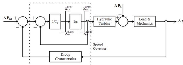
Figure 1. Block diagram of turbine, governor, load and machine
