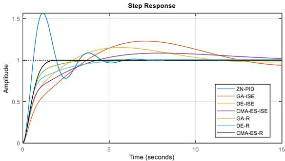
Figure 6. Time domain responses of the closed loop systems with the obtained controllers
