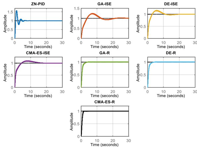
Figure 10. Time domain responses of the closed loop systems with the obtained controllers under parametric uncertainty
