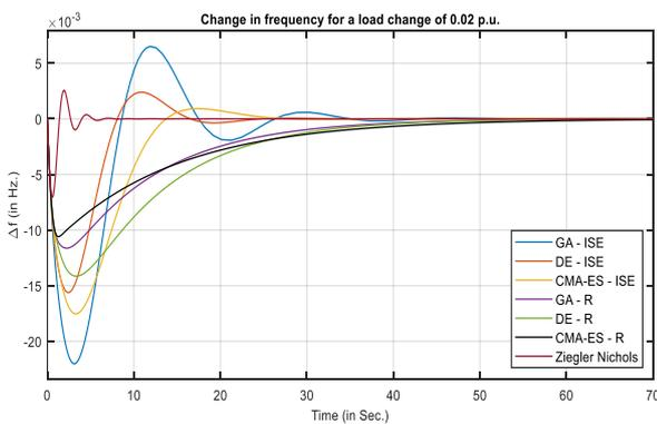
Figure 12. Time profiles of frequency after a load change of 0.02. p.u.
