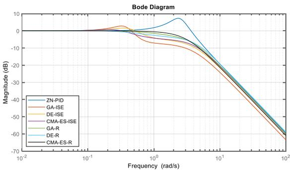
Figure 7 Frequency domain responses of the closed loop systems with the obtained controllers
