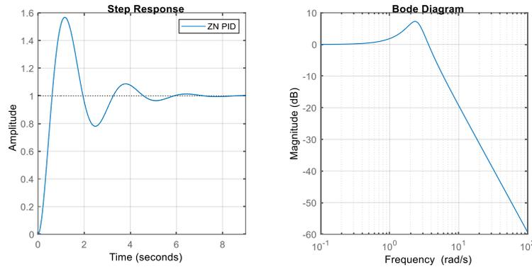
Figure 3. The time and frequency responses of the closed loop system with ZN-PID controller
