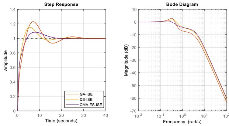
Figure 4. Time and frequency responses of the closed loop systems with controller gains obtained using GA, DE and CMA-ES by minimizing ISE
