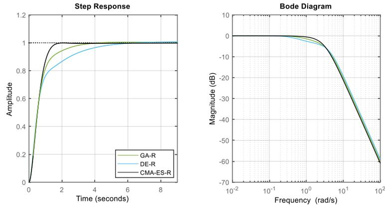
Figure 5. Time and frequency responses of the robust closed loop systems with controller gains obtained using GA, DE and CMA-ES
