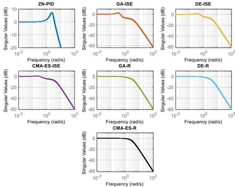
Figure 11. Frequency domain responses of the closed loop systems with the obtained controllers under parametric uncertainty
