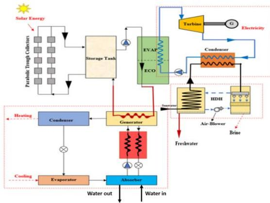
Figure 1. Schematic of solar-powered trigeneration arrangement for cooling, power, and drinking water generation
