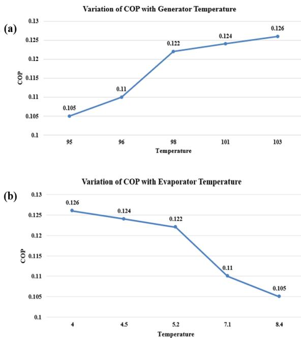
Figure 7. Variation of COP with (a) generator temperature, and (b) evaporator temperature
