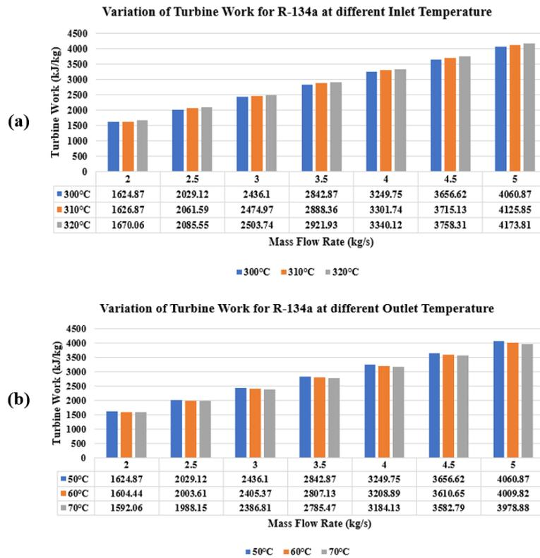
Figure 4. Variation of turbine work for R134a at different (a) inlet temperatures, and (b) outlet temperatures
