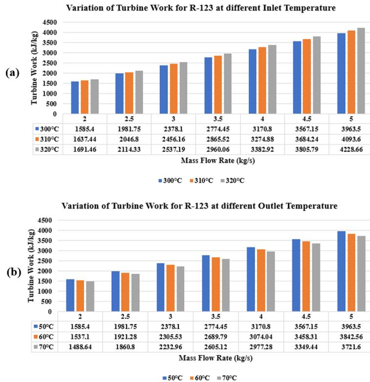
Figure 3. Variation of turbine work for R123 at different (a) inlet temperatures, and (b) outlet temperatures
