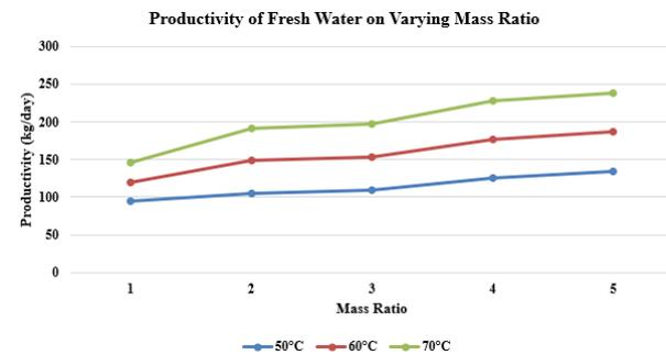
Figure 5. Production of fresh water on varying the mass ratio
