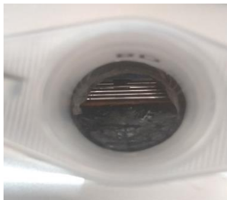
Figure 2. Syringe with razor blade setup (inner view). Commercial multi razor blade mounted on the cut portion of the barrel with blades assembly kept inclined inwardly.
