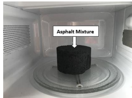
Figure 2. Stone mastic asphalt mixture sample in microwave
