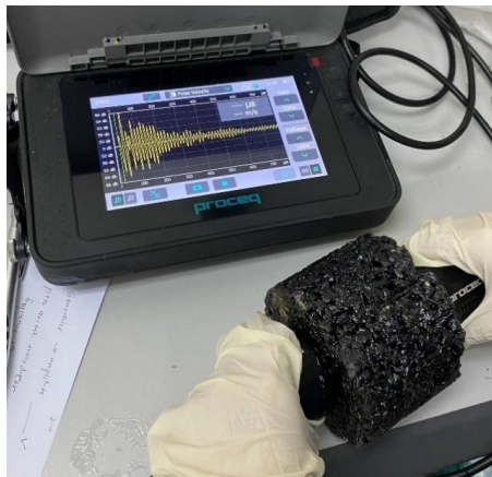
Figure 4. Ultrasound pulse velocity measurement setup
