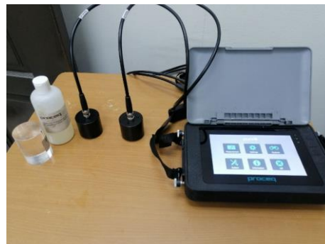
Figure 3. Ultrasonic Pulse Velocity (UPV) equipment used
