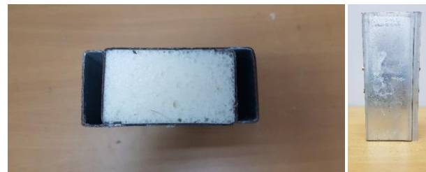
Figure 2. An example of the built-up slot-in CFS section filled with PF
