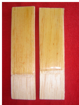
Figure 9. Coating film samples on plywood (2.5x8.0 cm) prepared from optimum formulation: ALNR, TPGDA and Irgacure 651 in ratio 100:80:10 by weight.
