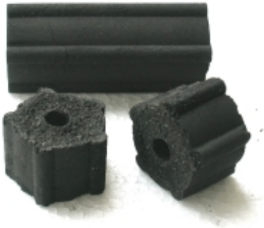
Figure 9. Schematic of Extruded fuel from the experiments.
