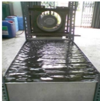
Figure 1. Pilot volatilization tank equipped with a wind generated system [Color figure can be viewed in the electronic version]
