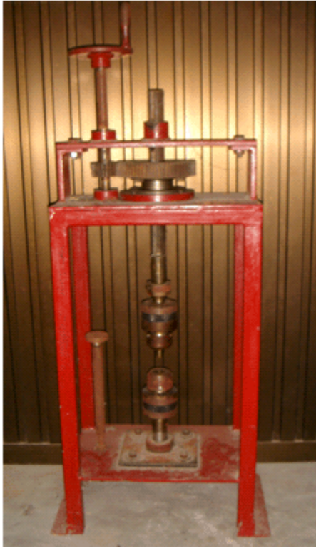
Figure 6. Control thickness of adhesive machine
