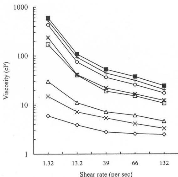
**Figure 7.** Effect of shear rate at various concentrations of exopolymers on the viscosity. The exopolymers were dissolved in distilled water (◇) 0.5%, (×) 1.0%, (Δ) 1.5%, (□) 2.0%, (\*) 2.5%, (○) 3%, (+) 3.5%, (■) 4.0%
