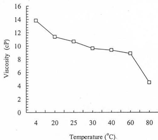
**Figure 8.** Viscosity of 2% exopolymers solution as a function of temperature. The solutions were measured at a shear rate of 100 rpm
