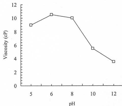
**Figure 9.** Viscosity of 2% exopolymers solution as a function of pH. The solutions were determined at 25°C at a shear rate of 100 rpm
