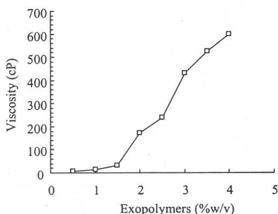
**Figure 6.** Viscosity of exopolymers at different concentrations. The samples were determined at 25°C at a shear rate of 1 rpm
