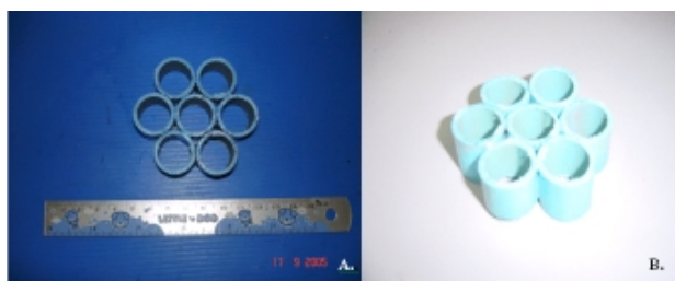
Figure 2. The microbial supporting materials in the UFAF reactor. (A) The top view (B) The side view
