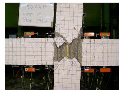
(c) Failure of specimen JS
