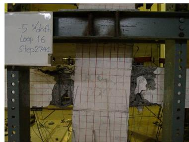
(a) Failure of specimen JL
