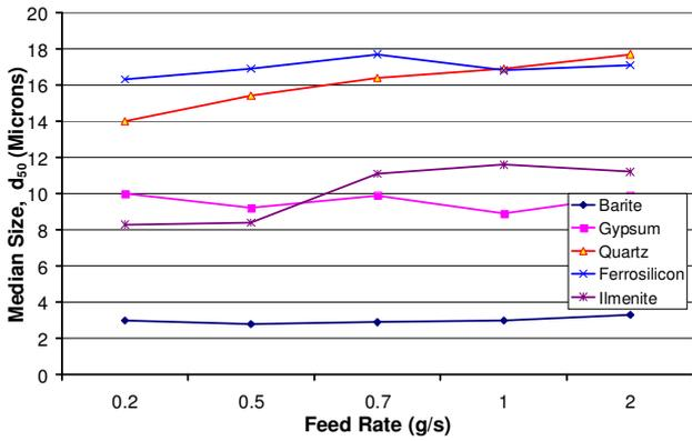
Figure 3. The variation of ground median size (d50) of minerals and material tested at pressure of 2 kg/cm<sup>2</sup> versus the feed rate of 297 microns feed size.
