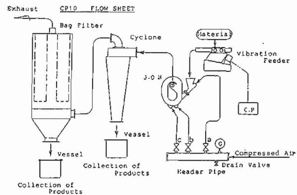
Figure 2. Illustration of a laboratory jet mill system (Seishin Enterprise, 1991).
