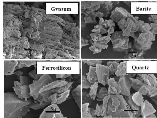
Figure 10. SEM images of ground gypsum, barite, ferrosilicon and quartz particles.
