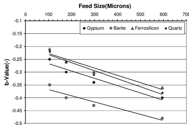
Figure 7. Relationship between b-value of an Equation (8) and feed size.
