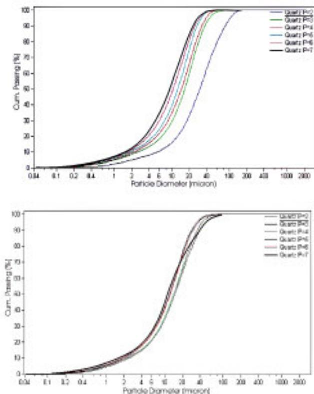
Figure 12. Particle size distributions of quartz ground products at a feed rate of 2 g/s, feed sizes of 595 (above) and 297 microns (bottom).
