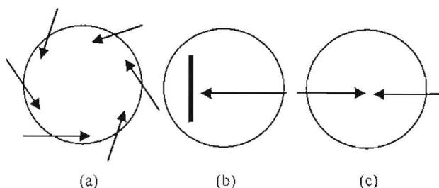
Figure 1. Principles of particle motion in 3 types of jet mill, a) spiral jet mill, b) target jet mill and c) opposed jet mill (Thaler, 2000).
