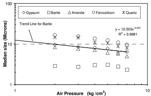
Figure 5. Correlations between the median sizes with air pressure of the ground materials at feed rates of 0.2~0.5 g/s and a feed size of 297 microns for different materials.
