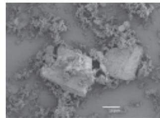
Figure 11. SEM image of gypsum ground product including blocks and platelets after milling at low pressure.
