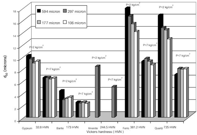
Figure 9. Relationship between  $d_{50}$  of ground products and the hardness of tested materials ground at various feed sizes and air pressures.
