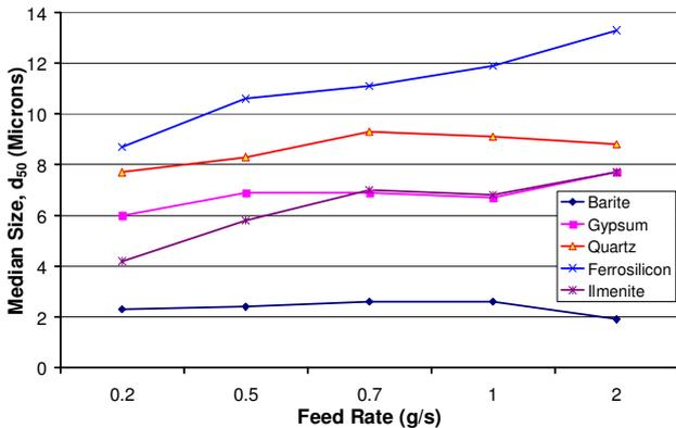
Figure 4. The variation of ground median size (d50) of minerals and material tested at pressure of 7 kg/cm<sup>2</sup> versus the feed rate of 297 microns feed size.
