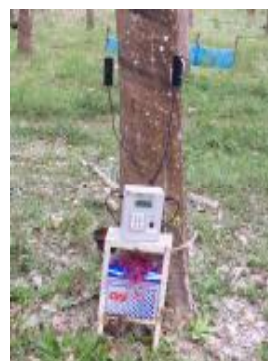
Figure 1. Installation of the sap flow sensors on the rubber tree in the experimental plot.
