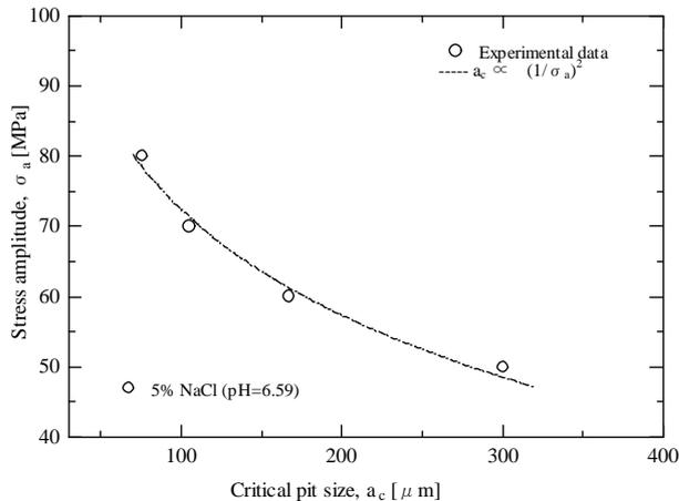
Figure 10. Variation of critical pit size with stress amplitude for AZ31 alloy under the NaCl environment.
