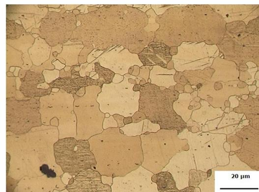
Figure 1. Microstructure of the AZ31 magnesium alloy.
