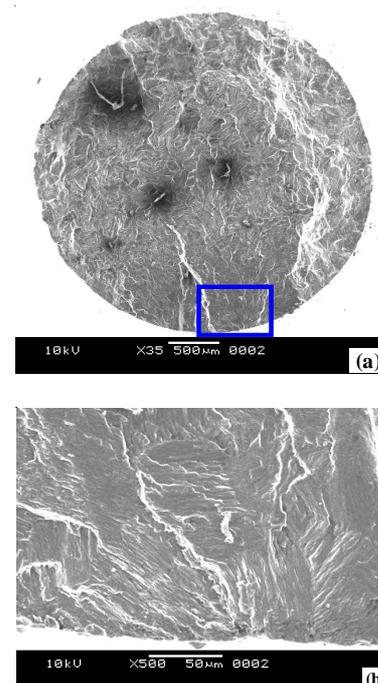
Figure 4. SEM fractographs showing (a) overall fracture surface, (b) magnified view of the crack nucleation region for the specimen tested at stress amplitude of 130 MPa under low humidity environment.
