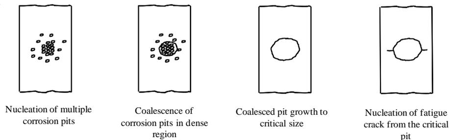
Figure 9. Schematic illustration showing the corrosion pit formation and growth of AZ31 alloy under the NaCl environment.
