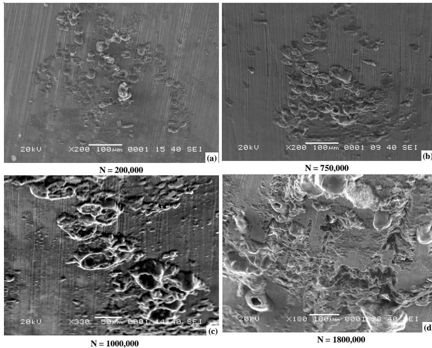
Figure 8. Specimen surface observations at the same location of the specimens tested under the NaCl environment at 50 MPa up to (a) 200,000 cycles, (b) 750,000 cycles, (c) 1000,000 cycles, and (d) 1800,000 cycles.
