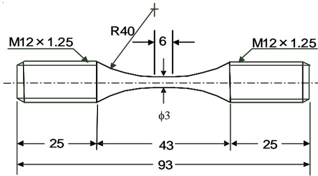
Figure 2. Shape and Sizes of the fatigue specimen.
