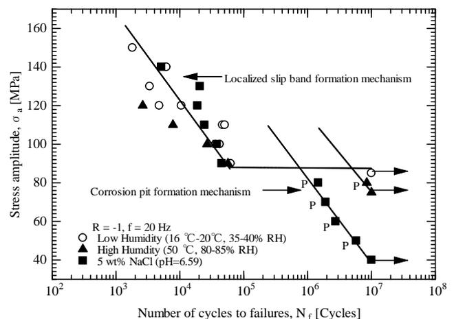
Figure 3. S-N curves for extruded AZ31 magnesium alloy under corrosive environments.
