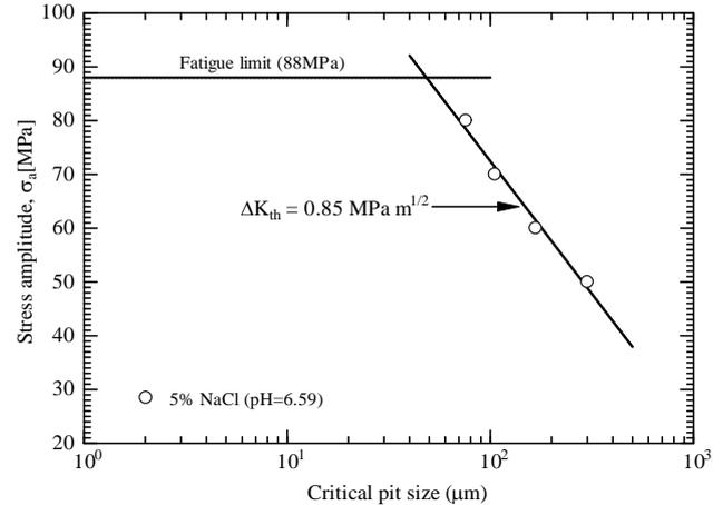
Figure 11. Critical pit size with stress amplitude for AZ31 alloy under the NaCl environment.
