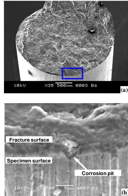
Figure 6. SEM fractographs showing (a) overall fracture surface, (b) corrosion pit at the crack initiation region for the specimen tested at stress amplitude of 80 MPa under high humidity environment.
