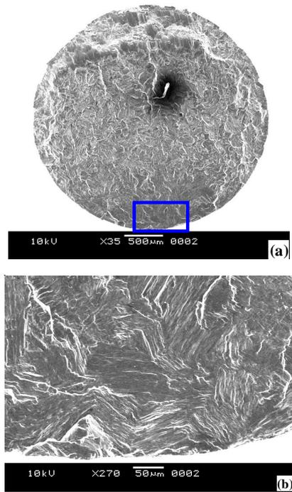
Figure 5. SEM fractographs showing (a) overall fracture surface, (b) magnified view of the crack nucleation region for the specimen tested at stress amplitude of 120 MPa.
