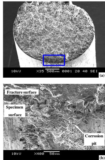
Figure 7. SEM fractographs showing (a) overall fracture surface, (b) corrosion pit at the crack initiation region for the specimen tested at stress amplitude of 80 MPa under the NaCl environment.
