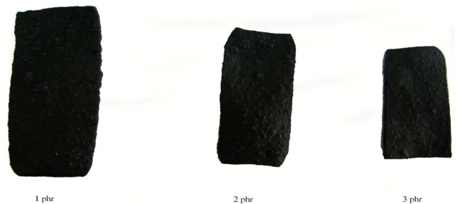
Figure 4. Photographs of WSR at various TBBS contents with SAP 40 phr, ZnO 3 phr, S 0.5 phr, carbon black 10 phr, and a soaking time of 91 days.
