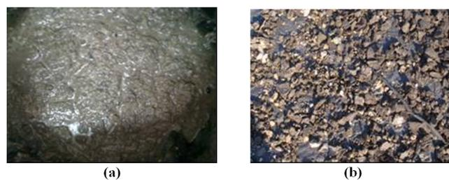
Figure 2. Trap grease used in the study; (a) before pre-treatment and (b) after pre-treatment.
