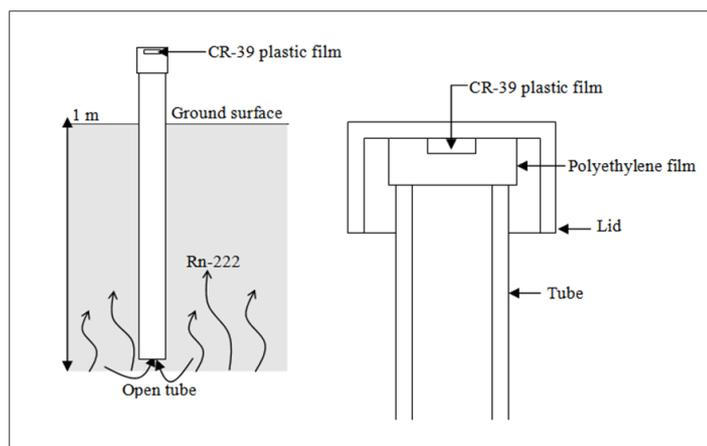
Figure 2. Schematic sketch showing the soil gas radon detection system.
