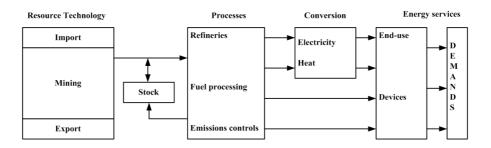
Figure 3. Schematic diagram of MARKAL-Thailand building blocks.
