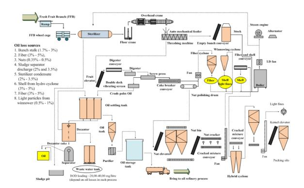
Figure 1. Selected large POM technology with wet exaction process.
