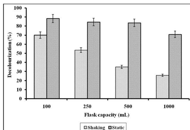
Figure 1. Influence of shaking and static condition and reaction flask volume on AR-119 bioremediation (Dye containing medium 100 mL).
