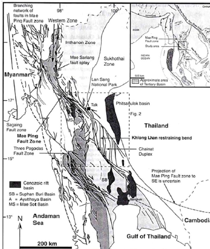
Figure 1. Three Pagodas strike-slip fault zone (TPFZ) of the west and central Thailand in relation to the regional tectonic setting, after Morley *et al.* (2007).
