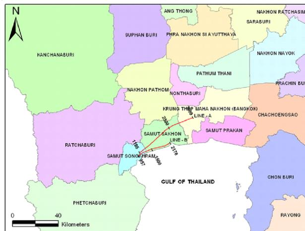
Figure 5. Two seismic lines acquired by Britoil Plc. in 1986 along the western part of the upper gulf of Thailand: Line A extends approximately 85 km long from Bang Khen through Bang Khae to Samut Song Khram, and Line B is approximately 40 km long from Samut Sakon to Samut Song Khram Province.
