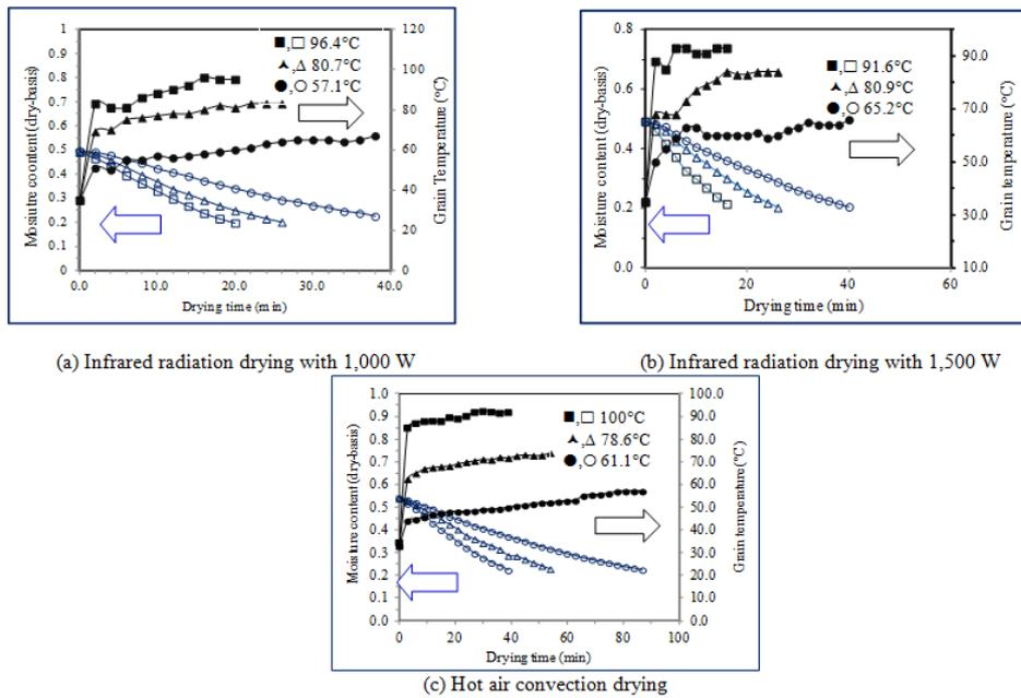
Figure 4. Moisture content and grain temperature against drying time of Suphanburi 1 (SP 1) parboiled rice drying with (a) IR 1,000 W, (b) IR 1,500 W and (c) hot air among inlet drying temperatures of 57.1-100°C
