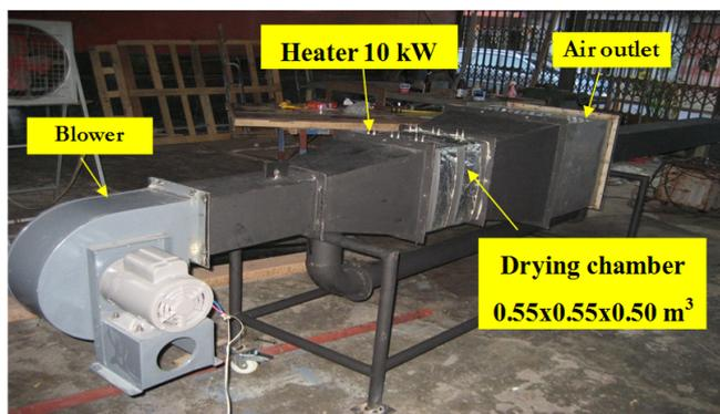
Figure 1. Illustration of tray drying system (PSU-TRD-08 2)
