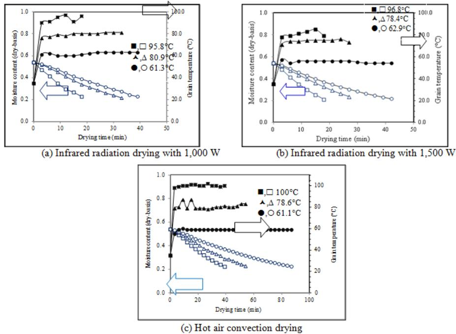
Figure 3. Moisture content and grain temperature against drying time of Leb Nok Pattani (LNP) parboiled rice drying with (a) IR 1,000 W, (b) IR 1,500 W and (c) hot air among inlet drying temperatures of 61.1-100°C
