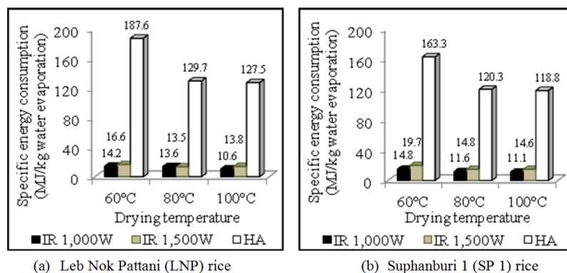
Figure 5. The specific energy consumption of parboiled rice drying versus drying temperatures of 60-100°C (a) Leb Nok Pattani rice and (b) Suphanburi 1 rice variety
