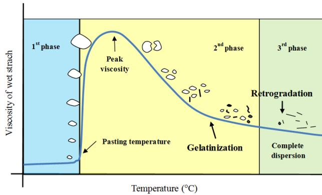
Figure 2. Illustration of viscosity property using rapid visco analyzer (RVA) [Adapted from Klanarong and Karlkule, 2003]
